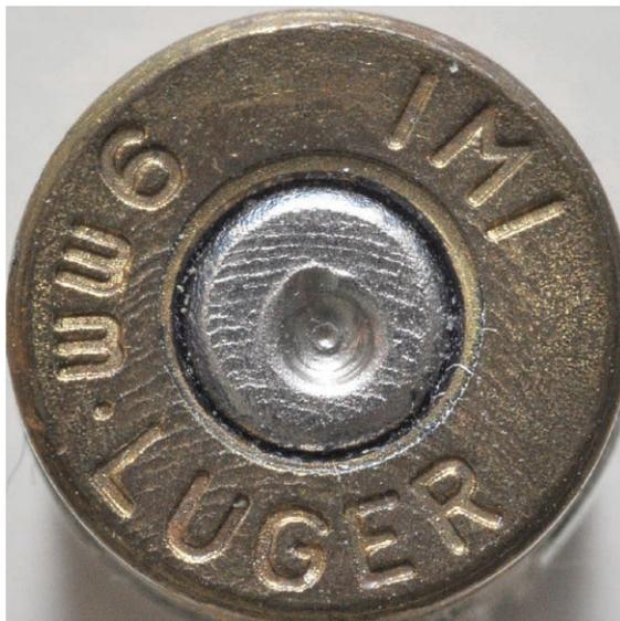
**Fig. 1.** Marks on the cartridge case discharged from FN HP-35 pistol
